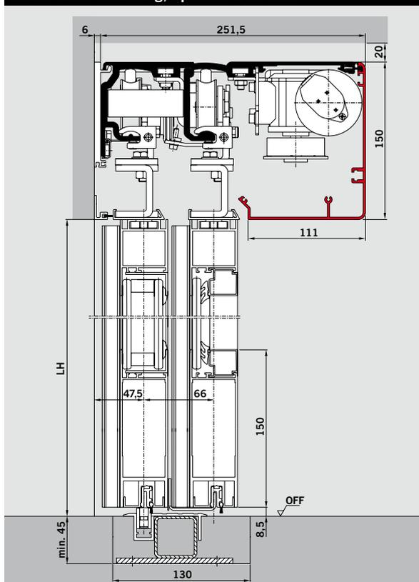
Horizontal section of connection profile for door systems that open only to one side
